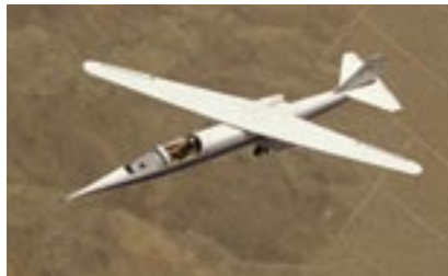
OBLIQUE WING Wing could be rotated for maximum efficiency
